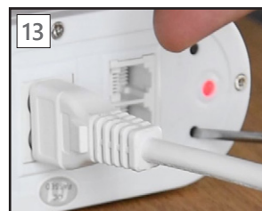
Turn on pairing mode on motor (Refer to the motor manual for how to enter pairing mode)
